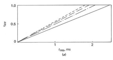
Influence of turbulence on evaporation rate-controlled combustion efficiency for three levels of pressure, D = 60μm (a) P=0.1MPa, (b) P=1MPa, (c) P=3MPa) (Fuel: Kerosene)
